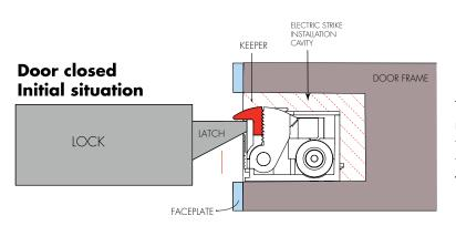
To understand the latch guide purpose, it is necessary to observe the latch movement when the door is about to be opened or closed. So, the following picture shows the initial position when the door is closed.
