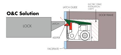
Thanks to the latch guide feature in the mini electric strike, the door won't be blocked. The latch is going to slide along the latch guide without getting stuck in the strike installation cavity.
